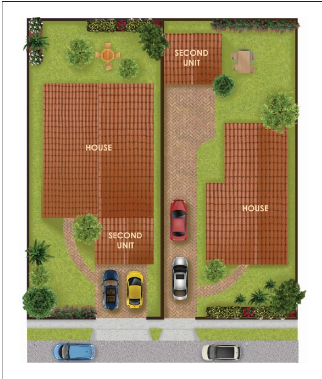
Figure 1. Garages converted to second units at the front and back of houses.
